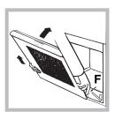
3. Grip the door on the two external sides and close it approximately half way. Unlock the door by pressing on the clamps **F**, then pull the door towards you lifting it out of its seat (see diagram).
